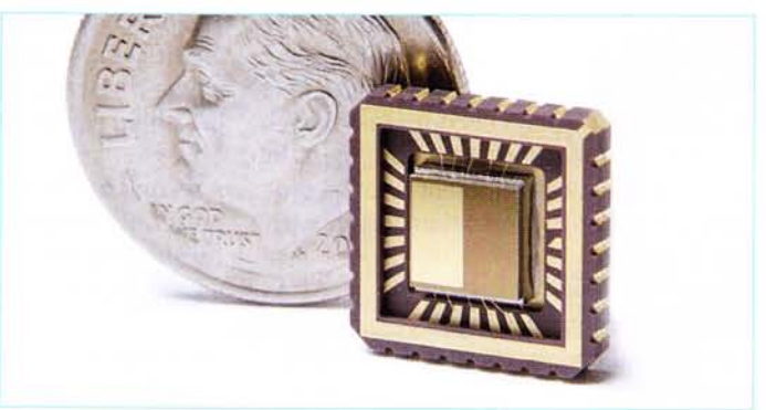
Figure 11. The SensorChip-CO 2 is a MEMS chip for measuring CO 2 (photo: ICX Technologies).
